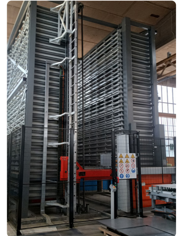
Automated storage system for metal sheets on trays
